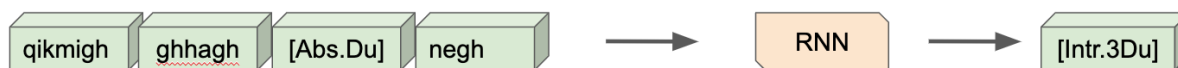
Figure 7.1: A recurrent neural network language model over morphemes can be used to predict the next morpheme in a sequence. In this figure, the light green boxes represent Yupik morphemes from Example (4), each encoded as a vector.
